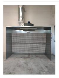
Example of paint cabin installation with extensions and roof, complete with lights and electrical panel.
