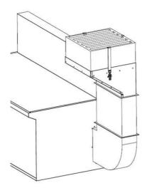
Exhaust kit with integrated HEPA 13 filter compatible with SBV benches.
