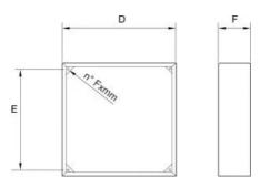
Rectangular spacer for fixing on thin walls for SEQ model fans.
