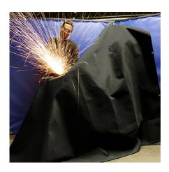
TOP series blanket recommended for a horizontal type of protection and therefore of incandescent material can fall and cool on it without puncturing it. In fact, Thetis weighs 1100gr/sqm and is 1.4mm thick and also undergoes a treatment on both sides based on Graphite (black) that raises the resistance temperature up to 700°C with peaks for short periods up to 900°C.
