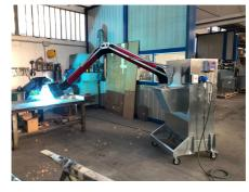
The DFC mobile wheeled fume and dust extractor is designed for the extraction and filtration of even very fine and volatile fumes and micro-dust generated during surface treatment processes of metals or composite materials.
