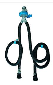
The GSW2T575 series wall-mounted extract or fan is a simple and economical solution for extracting exhaust gases from motorbikes or small/medium sized vehicles, when these are stationed indoors but it is necessary to keep the engine running for technical tests or temporary stationing
