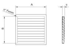
The SEQ axial fan gravity damper prevents heat loss when the fan is stopped, rain, wind and bird entry.
