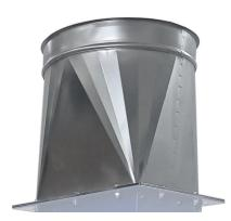
**Circular galvanized steel fitting**, complete with flange with borings for fixing to on fan discharge and beading prepared for collar on plant piping fixing side.
