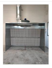
WFPN spray booths are equipped with integrated dry filtration and exhaust fan and due to their geometry form a constant speed suction front so as to capture pollutants produced by operations such as painting, resin coating, gluing and in all those professional treatments that generate application overspray.
