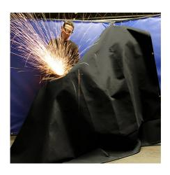
Blanket model BASIC made of fiberglass with polyurethane on one side, which has the only task of holding the glass fiber together, which otherwise will fray easily. This series is recommended for vertical protection in anticipation of a low amount of sparks and splashes.
