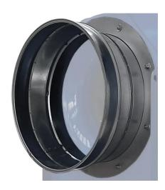
Circular suction fitting for SVM-R-F fans made of galvanized steel, complete with flange with holes for fastening to on fan suction and beading prepared for collar on plant piping fastening side.
