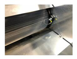
Replacement filter kit for installation of antistatic cartridges on DFC11 purifiers
