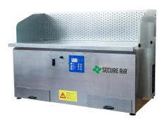
The SBC suction bench is available in 4 different sizes ranging from 1 to 3 meters. Designed to suck fumes and dust during professional operations that produce emissions dangerous for operators and the working environment as very volatile. This version is suitable for intensive use thanks to cartridge filters with compressed air cleaning, which ensure the restoration of maximum filtration efficiency at the end of the cycle and a long life in times.
